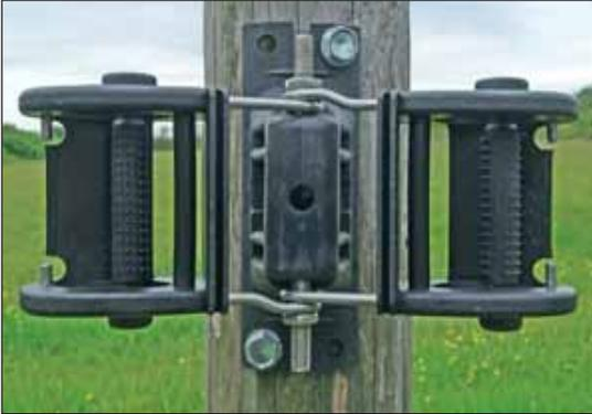
Step 1 : Screw the #BP37 with 2 lag bolts on wooden post or a hose clamp on metal post.
