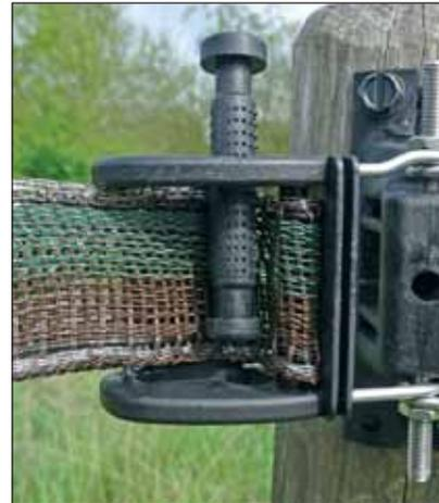
Step 7 : insert the pin roller at the front of the 2 layers of tape.
